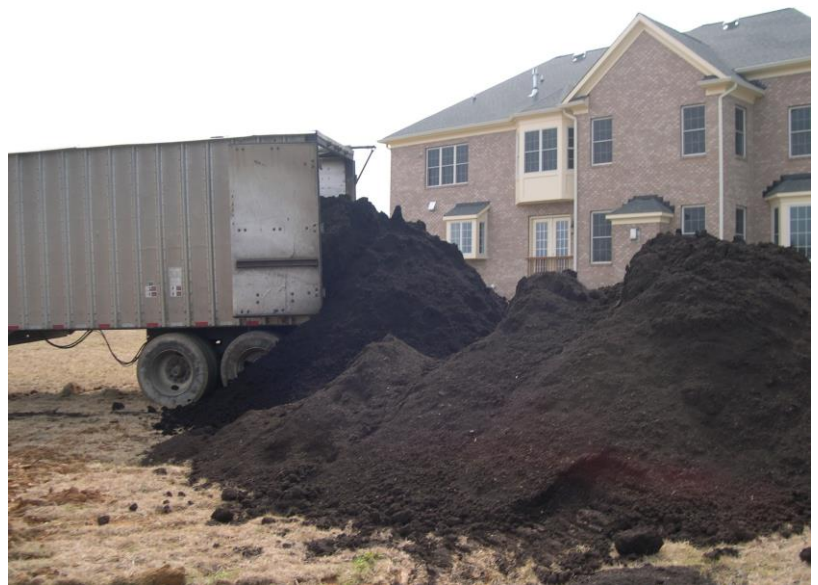
A walking floor tractor trailer, which holds 35 to 40 cubic yards, is often used to deliver compost to large job sites.
