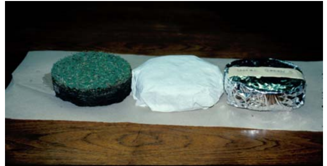
Cup cutter plugs (3.0 inch diameter x 2.0 inches deep) wrapped in a moist towel and wrapped again in aluminum foil are best.
